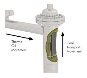
Preheating of coal with low-temperautre waste heat
