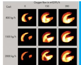
Improvement in the BF raceway obtained by PCI & OxyCoal+ at Dillinger Hütte AG, Germany
